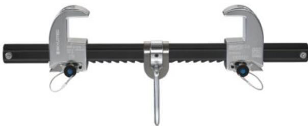
The BEAMTAC 2.0 mobile anchoring device is suitable for use as an attachment clamp for steel beams with a flange width of 90 to 380 millimetres and can be used for many different kinds of work in an industrial environment.
