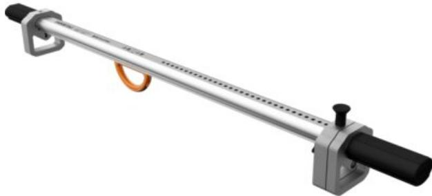
JAMBTAC Mobile Door Truss. Mobile anchoring point for all door widths from 600 to 1,100 mm. The adjustable mobile door truss made of aluminium is very light and can be easily adapted to different door widths. Rounded profile edges and plastic caps at the ends reduce the wear of material, the risk of injuries for the user and prevent the door posts from being scratched. JAMBTAC can be used simultaneously by up to two persons.
