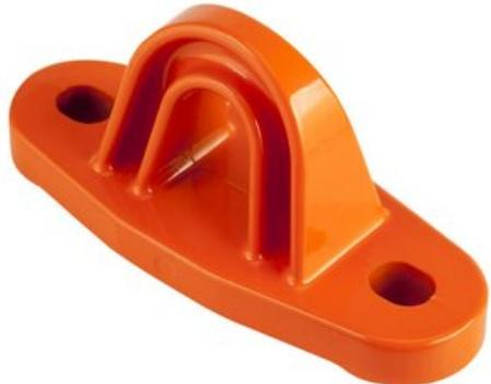
Fixed anchor points type AT 150. The anchor point is a connecting device mounted on a permanent structure. Installation on concrete with HST2 M12x115/20 Mounting Kit.
