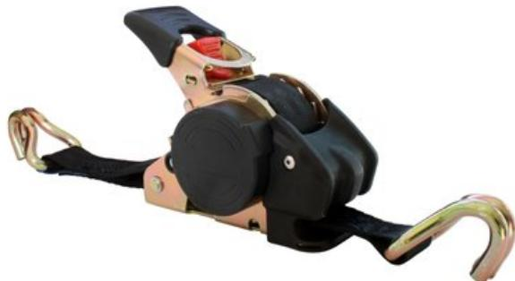
Rollo mini is a lashing for securing lighter cargo. Rollo mini is easy to use and the functionality is like a retractable seat belt. The lashing is rolled out to desired length and then tightened like an ordinary lashing. After usage the band retracts automatically. The lashing only consists of one part which benefits ease of use and simplicity.
